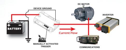
POWER-GATE Uni-directional relay can be manually activated or ignition-switched to power or de-power all high and low current accessories including motors, inverters, communications equipment, lighting, refrigerators/freezers, and sensitive computer equipment.
