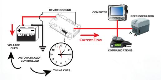
POWER-GATE Uni-directional relay can be programmed to automatically respond to low-voltage or high voltage battery conditions, and various timing cues making the device highly customizable. The ability to handle both high and low current in a single, easy-to-install module makes POWER-GATE a compelling choice when programmed to behave as a low voltage disconnect and preserve battery health.
