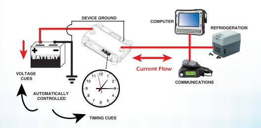
POWER-GATE Bi-directional relay can be programmed to automatically respond to low-voltage or high voltage battery conditions, and various timing cues making the device highly customizable. The ability to handle both high and low current in a single, easy-to-install module makes POWER-GATE a compelling choice when programmed to behave as a low voltage disconnect and preserve battery health.
