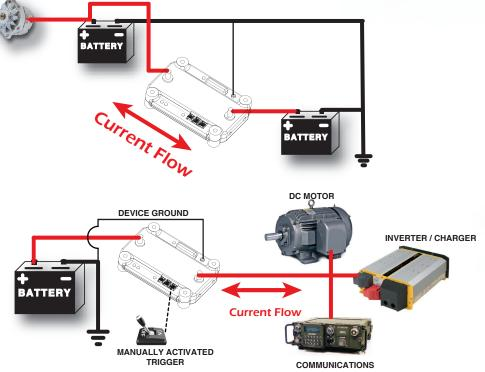
A Bi-directional relay must be used when voltage sources are present on both sides of the device in order to fully open the electrical circuit and insure no MOSFET damage occurs.
