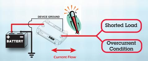
POWER-GATE Bi-directional relay can be programmed to respond as a precision circuit breaker. If the device senses a shorted load or an overcurrent condition, the device will "open" and de-power the output.
