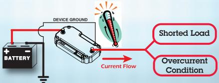
POWER-GATE Uni-directional relay can be programmed to respond as a precision circuit breaker. If the device senses a shorted load or an overcurrent condition, the device will "open" and de-power the output.
