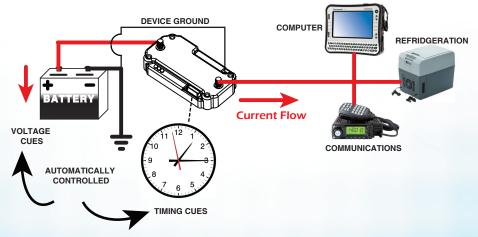
POWER-GATE Uni-directional relay can be programmed to automatically respond to low-voltage or high voltage battery conditions, and various timing cues making the device highly customizable. The ability to handle both high and low current in a single, easy-to-install module makes POWER-GATE a compelling choice when programmed to behave as a low
