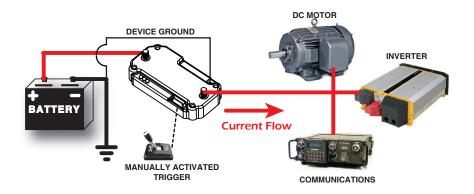
POWER-GATE Uni-directional relay can be manually activated or ignition-switched to power or de-power all high and low current accessories including motors, inverters, communications equipment, lighting, refrigerators/freezers, and
