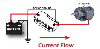
POWER-GATE Uni-directional relay must sit between a source and load. If a source of current is present on both the input and output of the relay, the bi-directional configuration is necessary.
