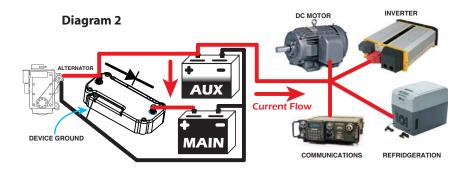
When the vehicle is off and load(s) are applied to the AUX battery, the AUX battery will discharge independent of the MAIN battery. Note the orientation of the diode symbol. The POWER-GATE's MOSFET array behaves like an "ideal" diode in that reverse current cannot flow from MAIN to AUX while forward current enjoys an absoute minimum voltage drop as denoted in Diagram 1.
