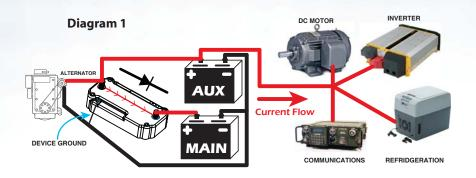
POWER-GATE Single Rectifier Isolator allows all batteries in the network to be charged. In Diagram 1, the alternator is charging the AUX battery which is common on the device input post, and current is flowing through the MOSFET array to the MAIN battery. All loads applied to both batteries are being powered. See Diagram 2 to see what happens when the AUX battery is discharged.
