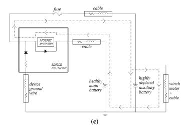
Figure 2: Reverse current turn-off transient behavior in combine mode with system loop inductance. (a) Main battery supplying current to depleted auxiliary battery and winch motor (diode functionality overridden). (b) Reverse current during MOSFET array turn-off. (c) Reverse current flowing through the MOSFET array protection circuitry due to system inductance.
